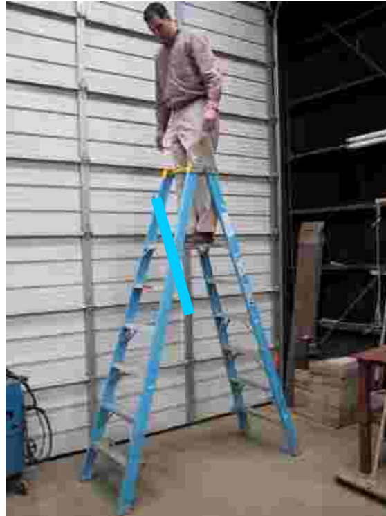
Figure 8 - A platform ladder and a double front ladder (Steps on both sides.)
