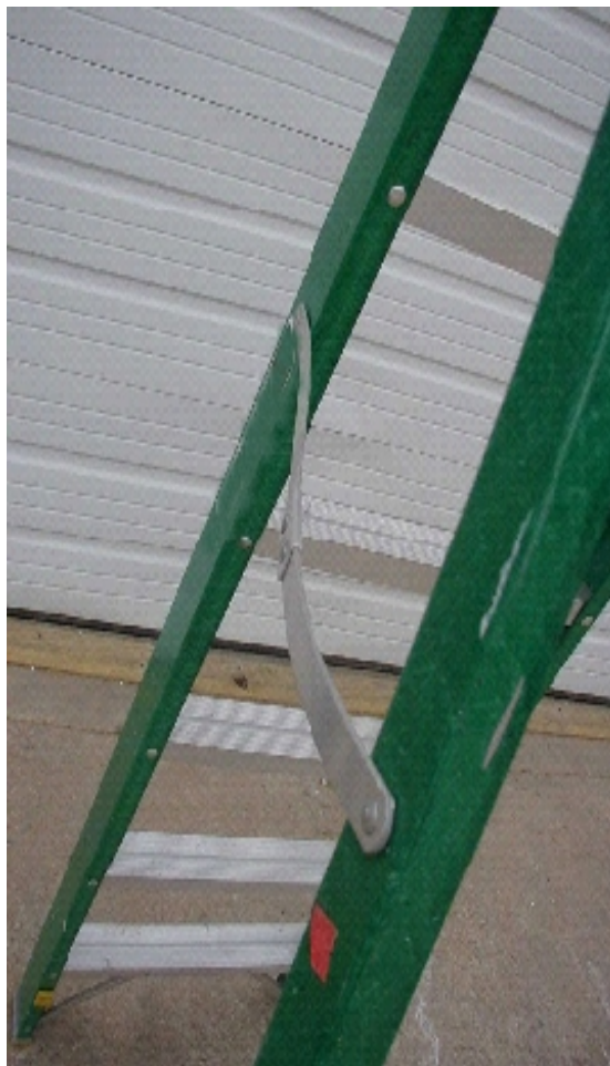
Figure 4 - Bent Spreader Bars Indicate Racking
