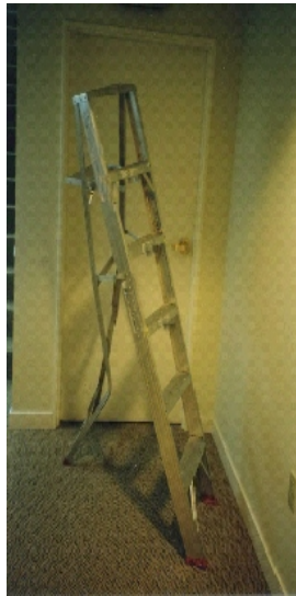
Figure 6 - Bent Rear Legs from Racked Stepladder
