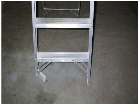
Figure 5 - Lower Front Leg Bent Inward Indicates Possible Stress Overload from Racking
