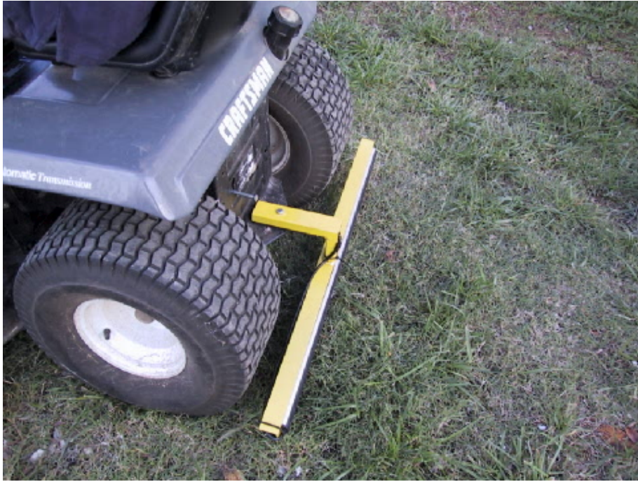
Figure 24: Side view of rear collision detector bumper
