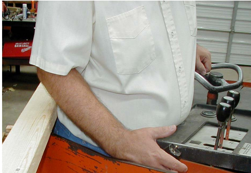
Incomplete guarding of the operator workspace can result in collision accidents
